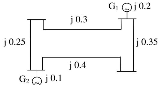
2. Obtain  $Z_{Bus}$  by using building algorithm for the following figure
