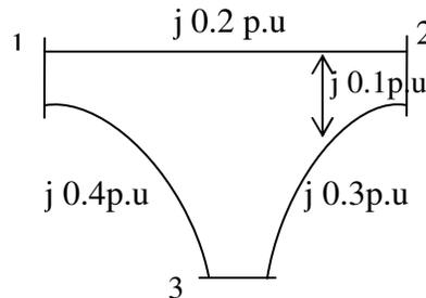
3. The power system network shown in below figure. Each line has a series impedance of  $(0.01+j0.06)$  p.u and the total shunt admittance of  $j 0.04$  p.u. The specific quantities of the buses are given in the figure. A controlled reactive power source is available at bus 3, with the constraint  $0 \leq Q_{g3} \leq 2.0$  p.u. Using gauss – seidel method, find the voltage at bus '2' and '3' after the first iteration.
