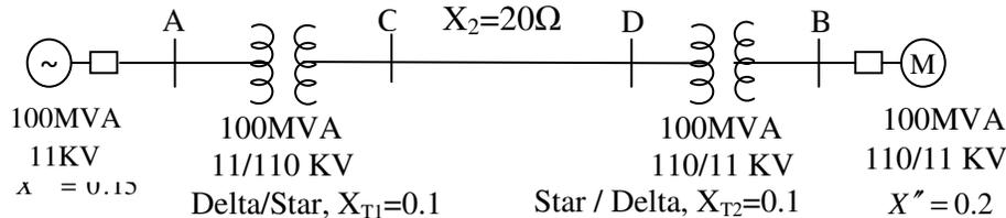
The synchronous generator is operating at its rated MVA at 0.9 p.f lag and at rated voltage. A 3-phase short circuit occurs at bus 'A', calculate p.u value of (i) sub transient fault current (ii) sub transient generator and motor current. Neglect pre-fault current. Also compute (iii) sub transient generator and motor currents including the effect of pre-fault currents.
